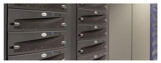
7. The high speed fibre optical storage array.
