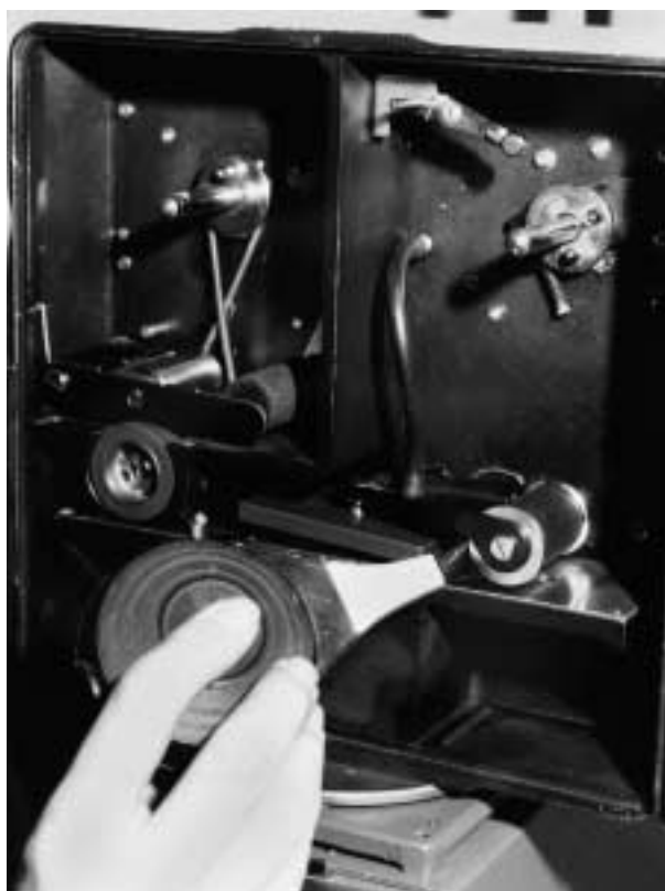
Cleaning a camera head with a brush
