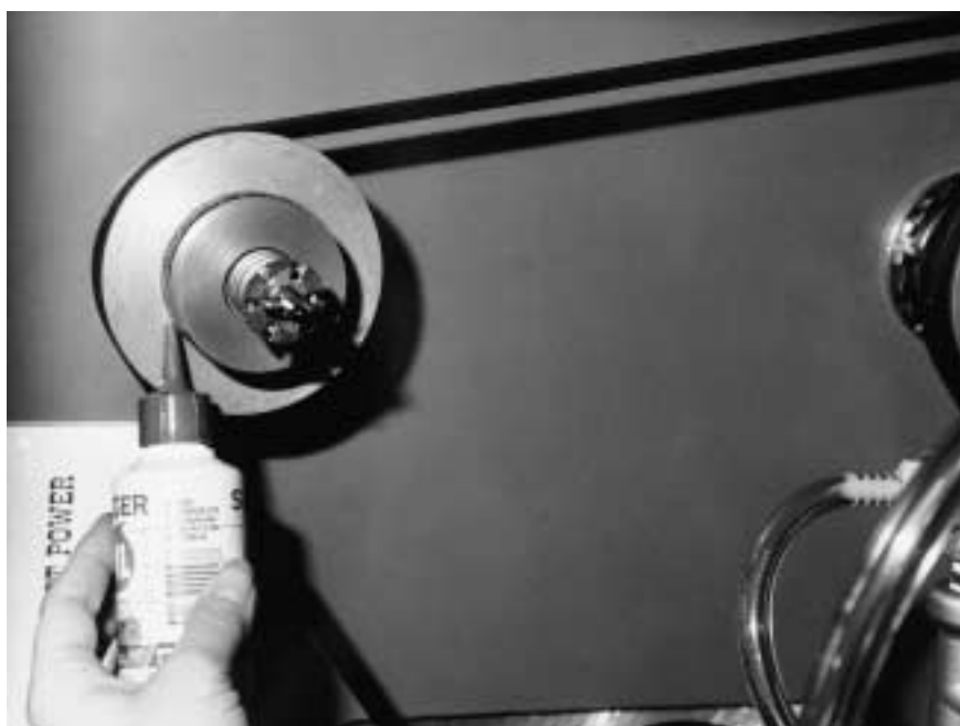
Lubrication – oiling the pads of the duplicator
